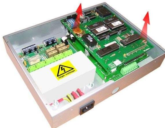
Mounting the NMU, use the template to pre-drill the wall to mount the NMU in the desired location. Screw the NMU to the wall at the four points indicated above. Ensure that the location has enough clearance around the NMU to allow the fitment of the lid retaining screws and any cable exits.
