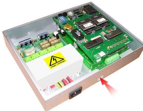
Remove the Processor Board. Remove the four M3 screws that locate the processor board then remove it by carefully pulling towards you to disengage it from the 50-way connector.
